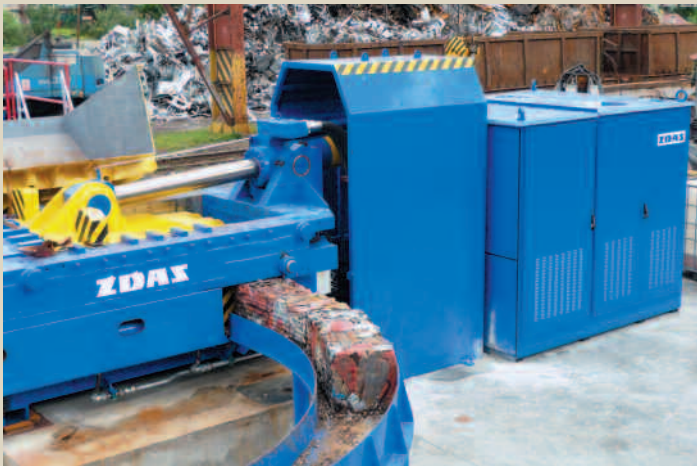
The press includes a bale conveyer
