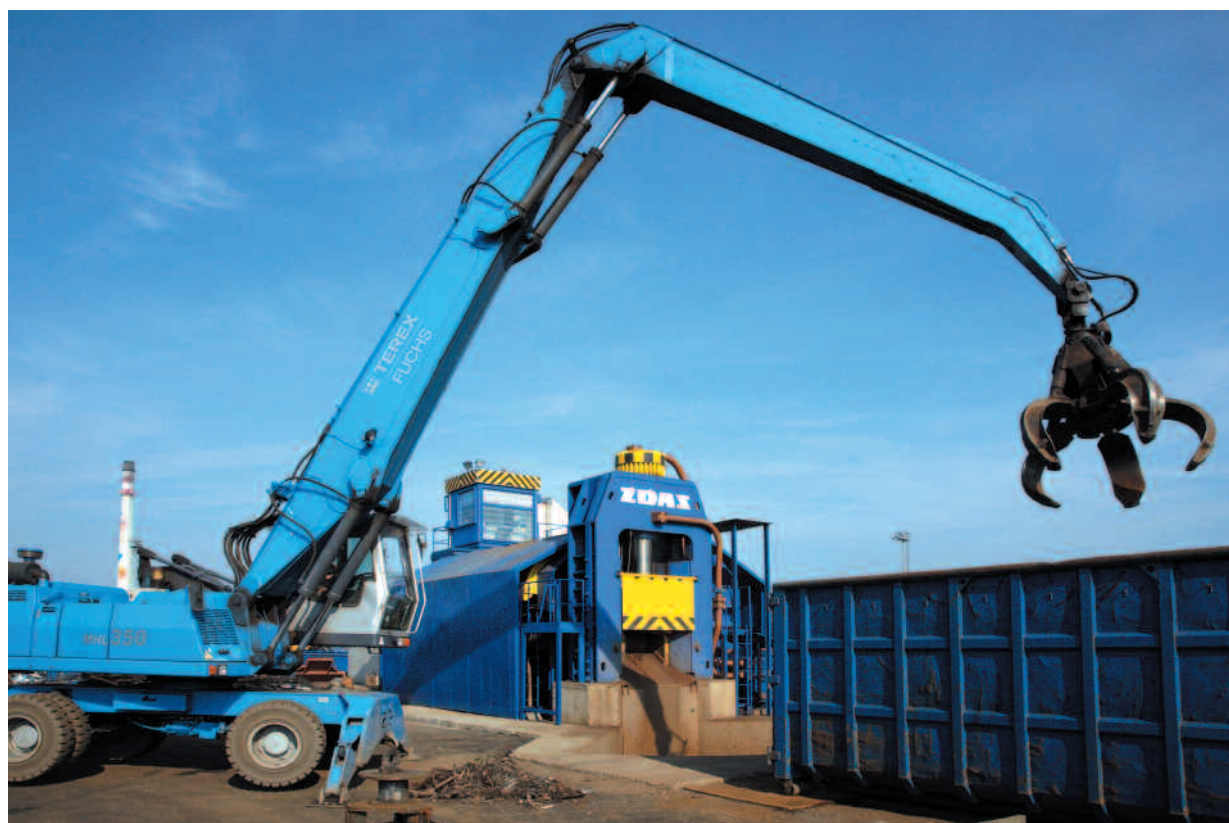
Workplace with CNS-PVM hydraulic shear
