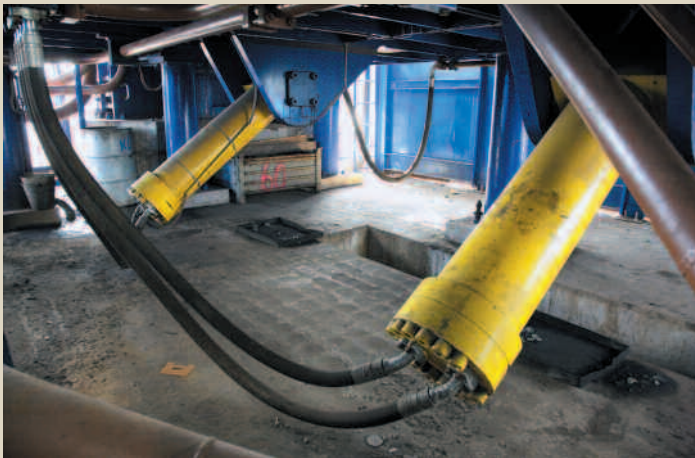
Hydraulic cylinders operating the folding cover
