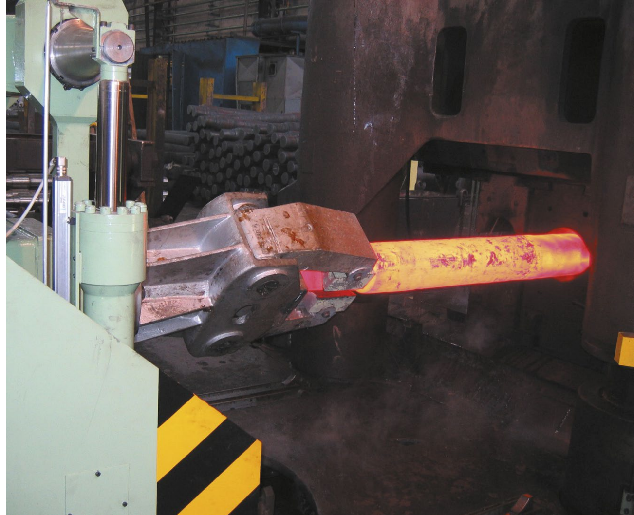
▲ Forged railway axle between the swages of a CKNV 1000 Press
