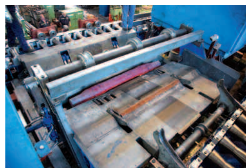
Railway axle in the straightening press
