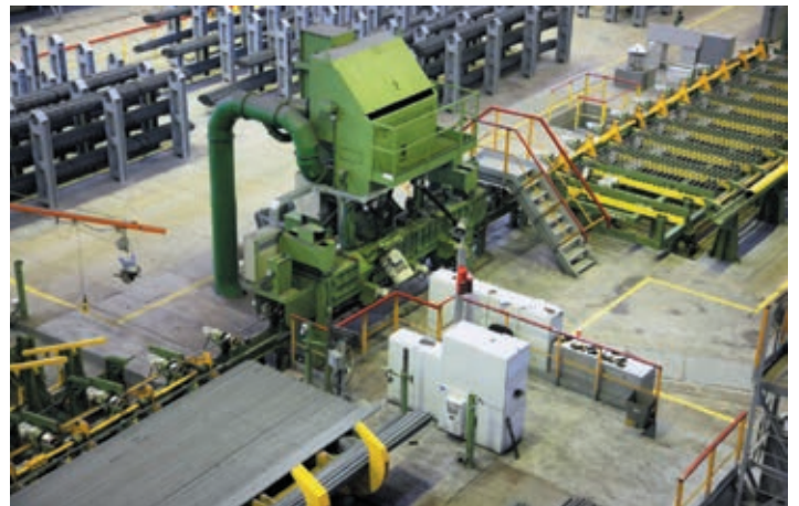
(2) Steel shot blasting of the bars
