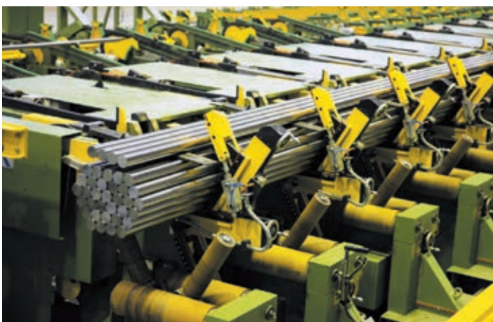
(10a) Bundling the bars together
