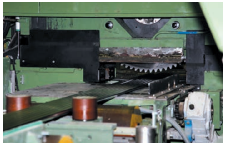
(6) Cutting bars to commercial lengths
