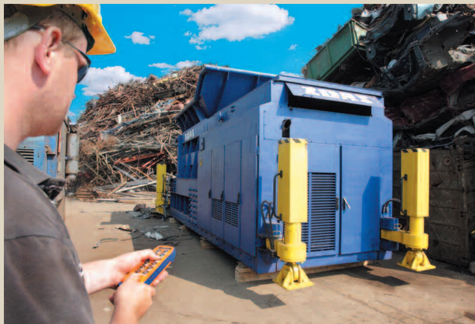
Remote control of the shears by the scrap yard operator
