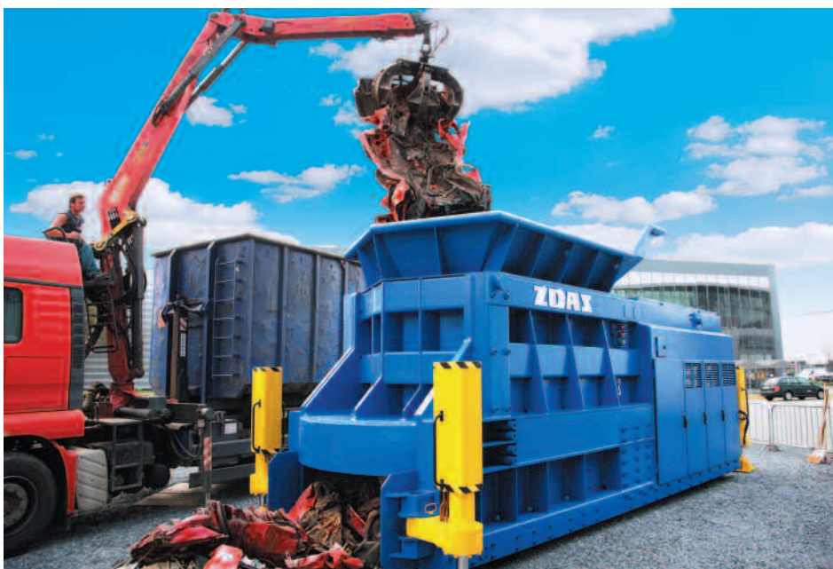
Loading scrap into the CNS 730/190 shears
