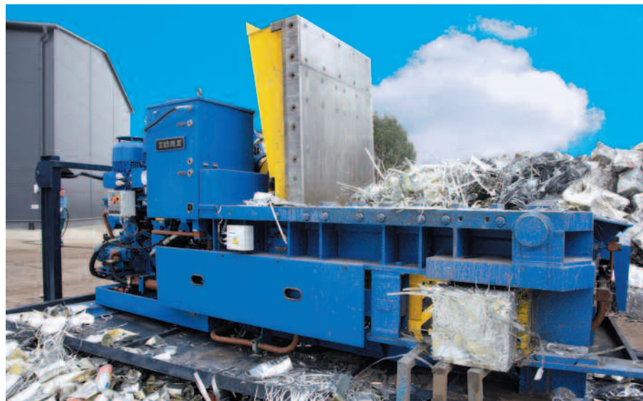
Opening the cover enables sufficient space for scrap feeding
