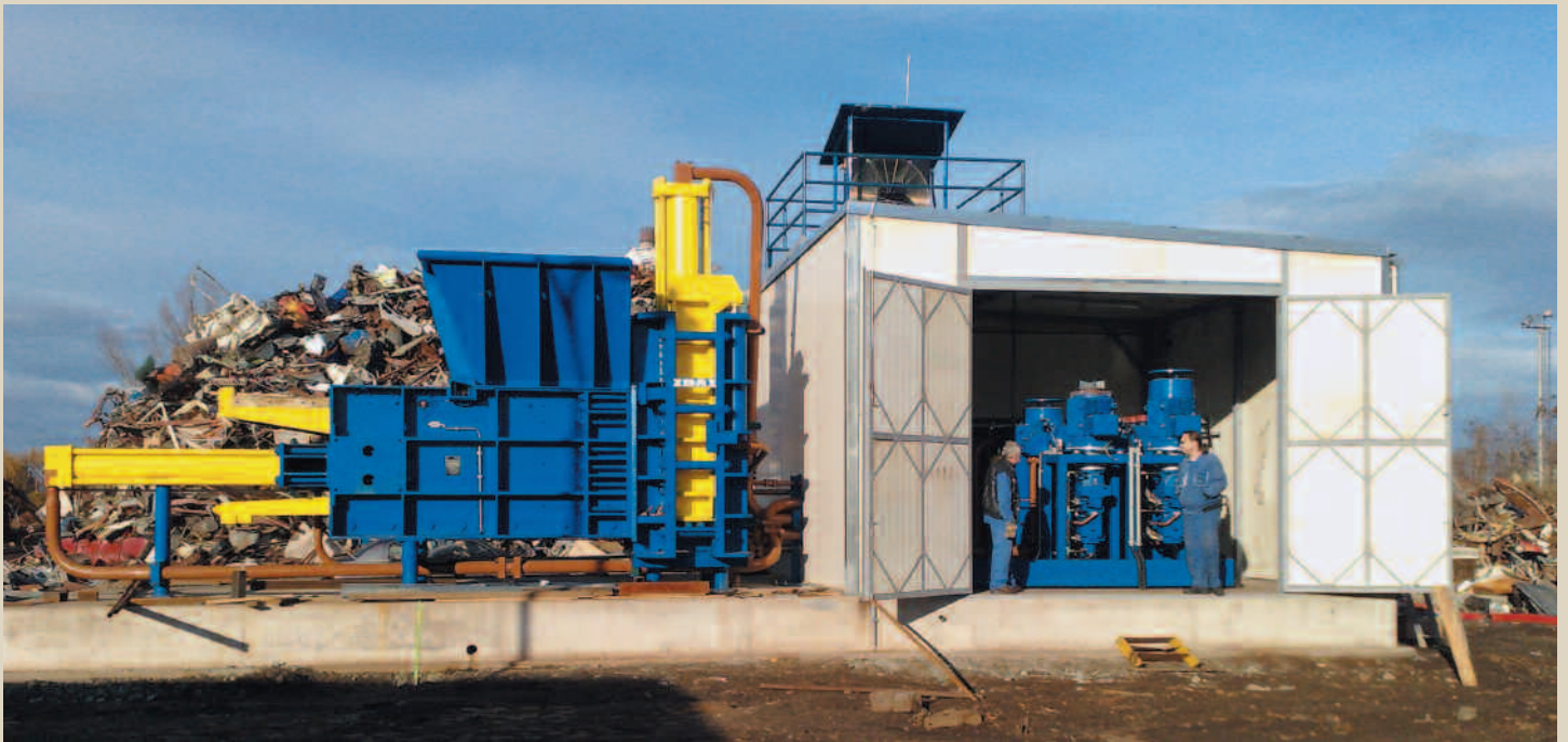
Press drive in a separate cabin
