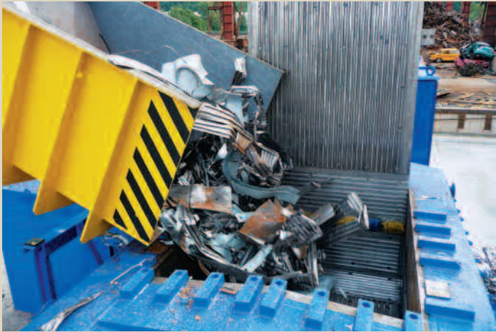
Tilting the hopper of the CPB 200 press enables easy scrap loading
