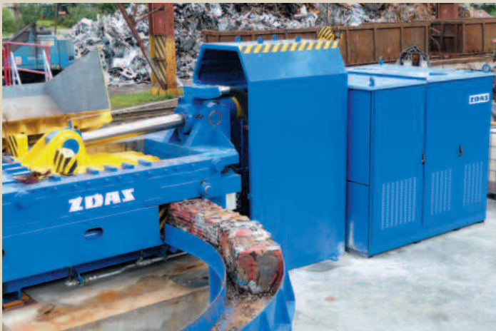
The press includes a bale conveyer
