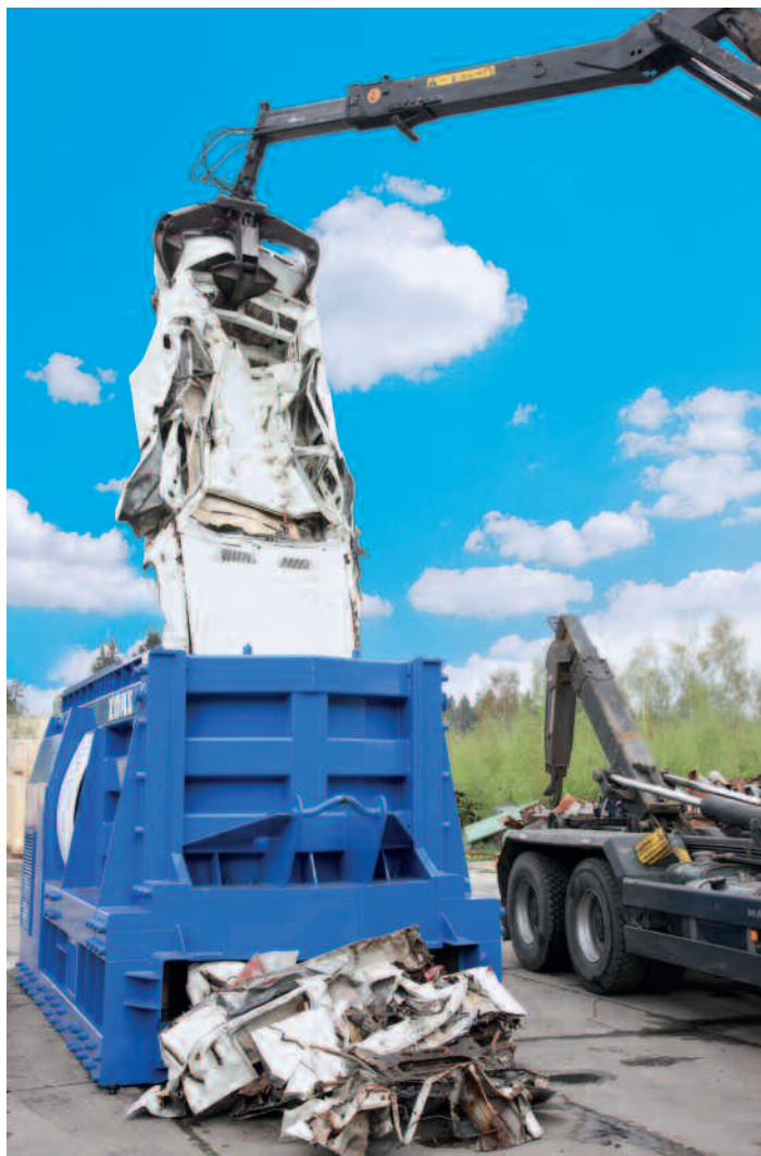
Loading the CNS 400 K shears with car scrap
