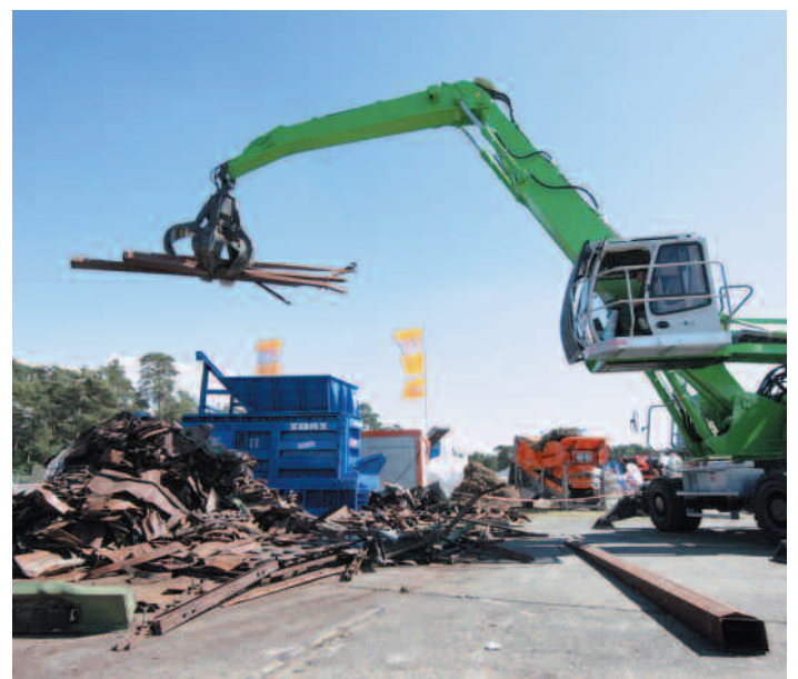
Loading the CNS 400 K shears with long scrap
