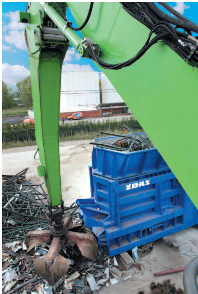
Loading the CNS 400 K shears with a grab loader
