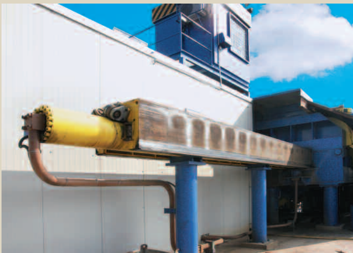
The pusher's hydraulic drive
