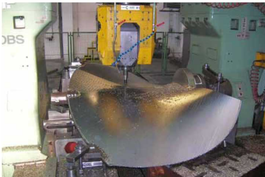
Kaplan turbine blade for ČKD Blansko Engineering
