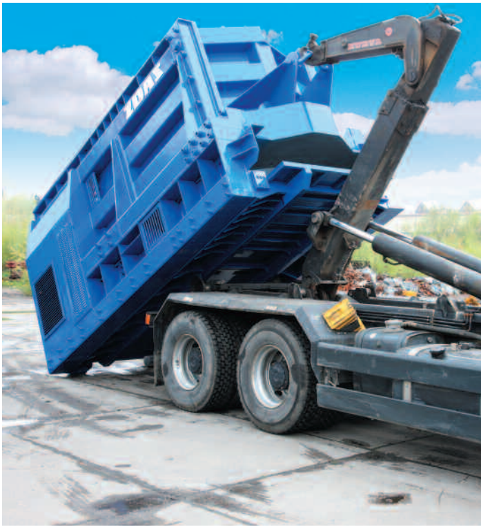
Loading the container shears on a carrier
