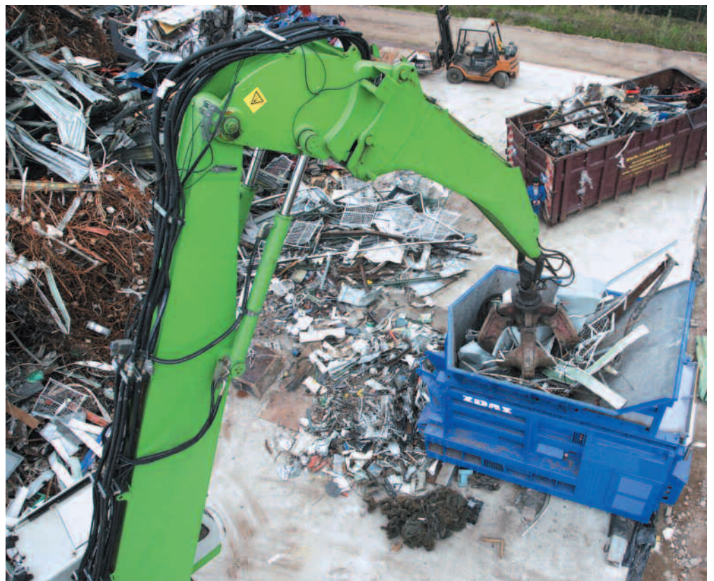
Layout of the workplace with the CNS 400 K shears
