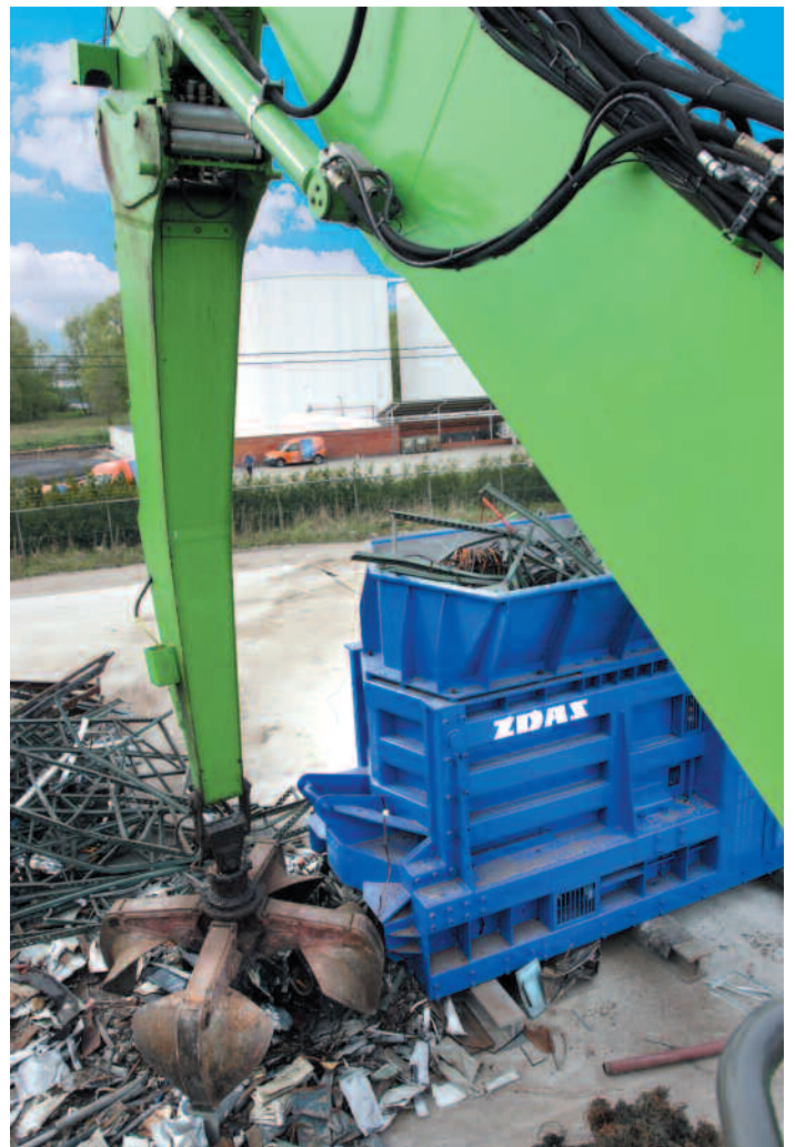
Loading the CNS 400 K shears with a grab loader
