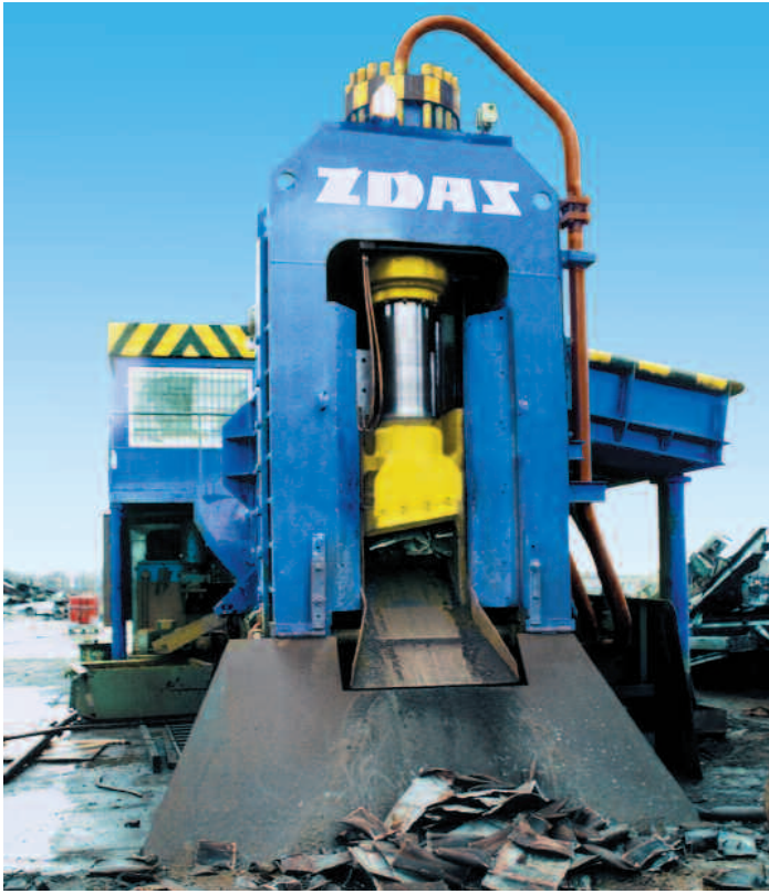
CNS 630-S wing shear is a stationary shear with high output
