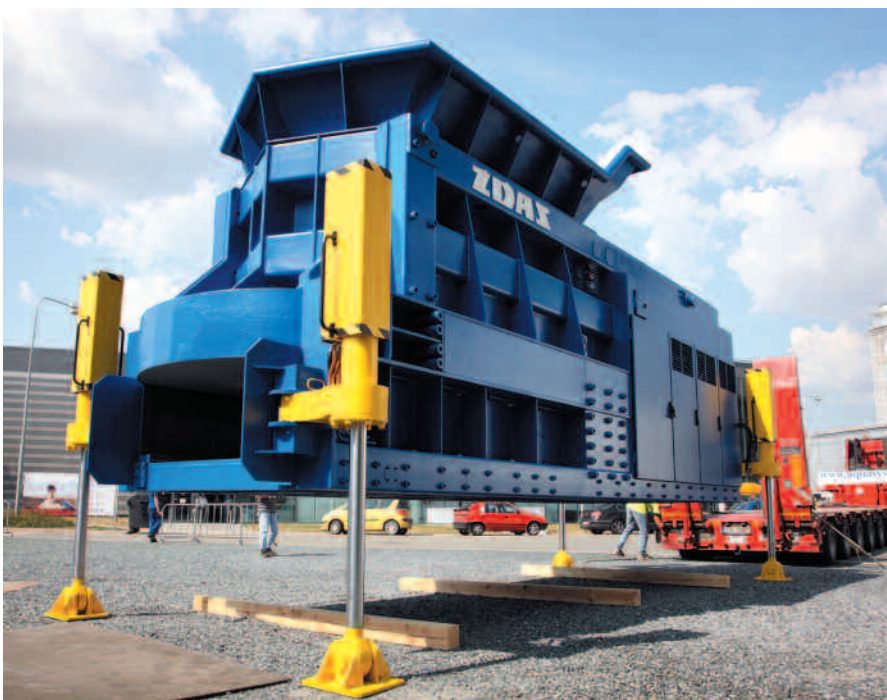
CNS 730/190 shear ready to be loaded on a flatbed trailer
