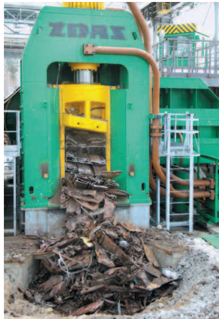
Pushing out the cut scrap
